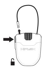
To unlock, adjust the code to be correct and press
