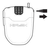
Release the reset button by removing pen
