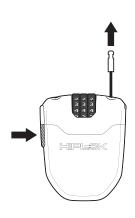
To release, ensure lock is on unlock code and press
