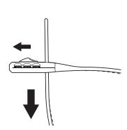
Push release button while pulling the tie out of the lock
